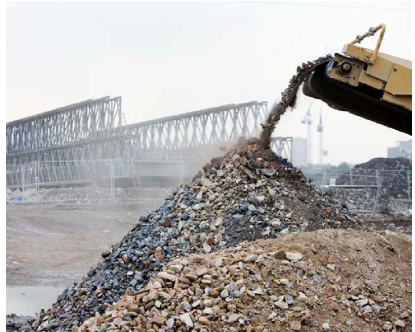
Conveyor belt on plant designed to reuse concrete from demolished buildings on the London 2012 Aquatics Centre site.
