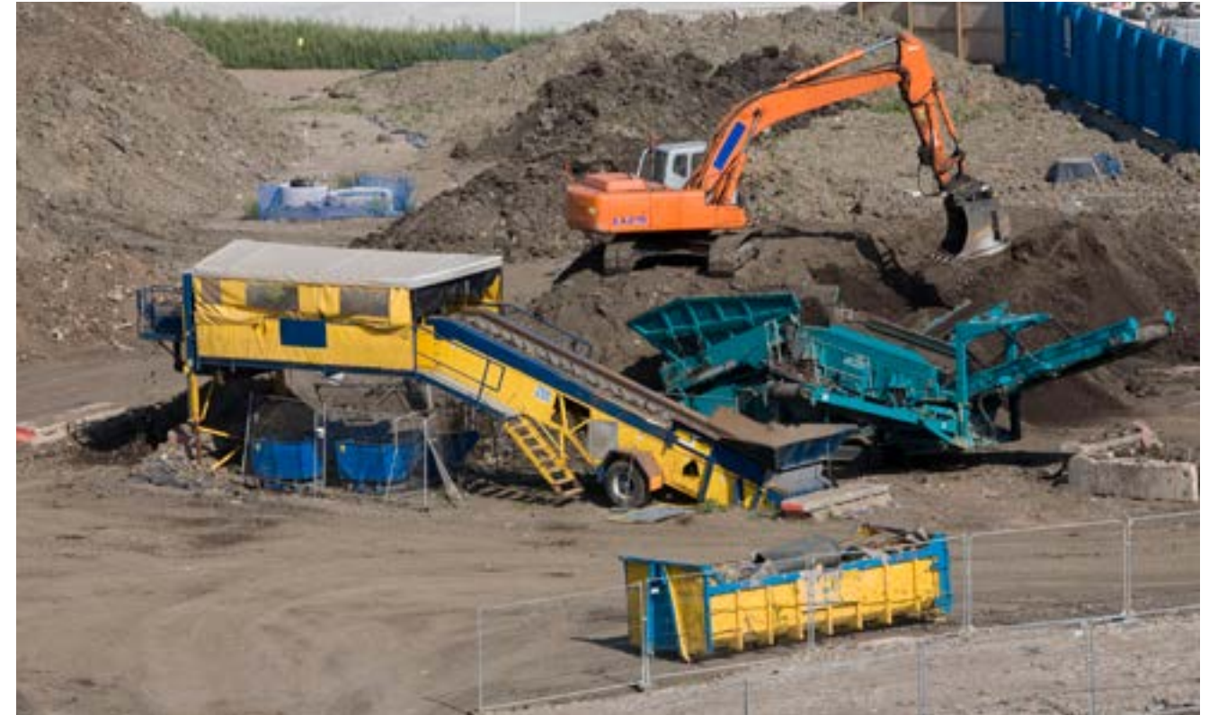
Complex sort machine on the London 2012 Velo Park. This machine cleans large waste materials from soil as part of the wider aim of bio-remediation and re-use of all the soil within the Olympic Park.
